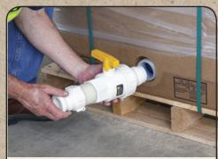
With the valve in the closed position begin threading the ball valve assembly into the dispense gland.
