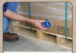
Remove the blue 2" plug from the dispense outlet. You will find a 2" crown cutter tool affixed to the back of the plug.
