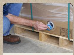
Separate the 2" crown cutter from the plug and reinsert it into the dispense gland with the "teeth" pointing toward the liner membrane.
