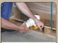
Continue threading the ball valve assembly clockwise into the dispense gland.
